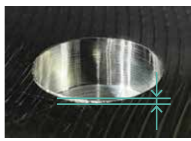
Cutting conditions: \phi 8.0 mm, 5xD, 42CrMo4, v_c = 90 m/min, f = 0.20 mm/rev, wet (internal supply)
